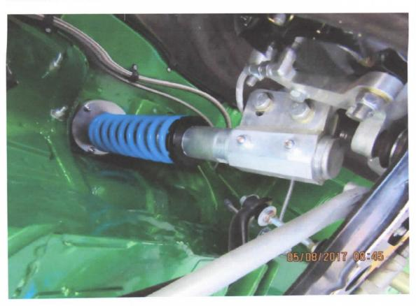
**Rear suspension** – Supplied by RRS Pty Ltd & fitted in accordance with manufacturers installation instructions.
