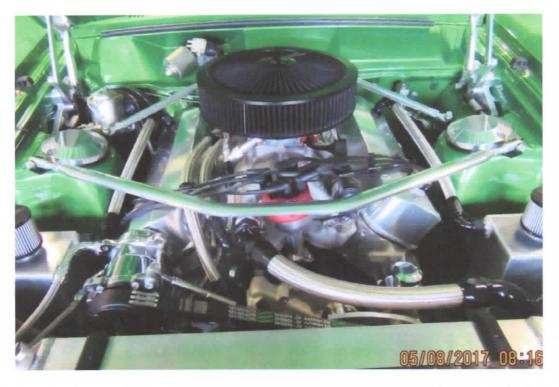
A OEM 460 cubic inch engine is fitted with a sports camshaft, optional alloy cylinder heads(Torino engine heads), alloy inlet manifold, Pacemaker extractors and a Holley 4 barrel carburettor. ADR 26 emission components connected.
